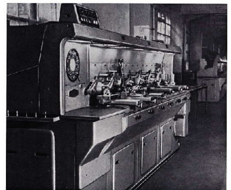
Automatic line installed at the 1st Moscow Horological Factory for machining watch cases.
