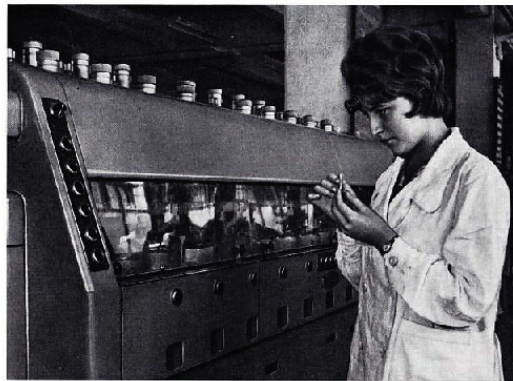
Automatic line installed at the 2nd Moscow Horological Factory for machining the plates of ladies' wrist watches of the "Slava" model. The line was also built at this factory.
